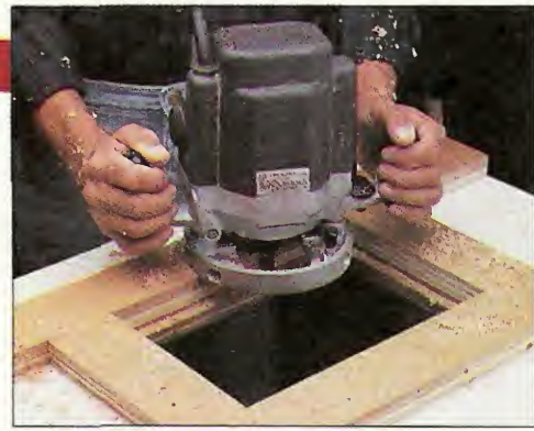
▲ Using a pattern bit in a router is a quick way to rout the recessed lip in the top. The bearing on the pattern bit rides against guide strips and cuts a recess exactly the same size as the insert plate.
