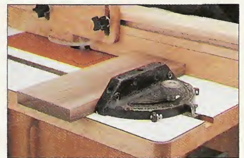
▲ A channel can be routed to accept your miter gauge. This is particularly handy for routing the ends of boards.
