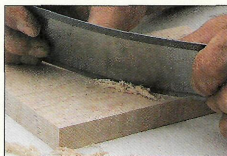
▲ Highly-Figured Grain. Smoothing highly-figured grain and burls is one area where a scraper has no equal.
