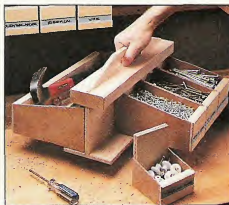
▲ Use this carrier to take bins and tools wherever they're needed. When not in use it fits in the rails on the wall.
