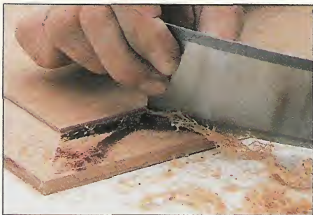
▲ Burn Marks. A hand scraper is the tool I reach for most often to remove stubborn burn and saw marks.
