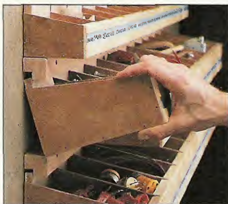
▲ The back of each bin "locks" into a wall-mounted rail. To remove the bin simply lift the front up and pull it out.
