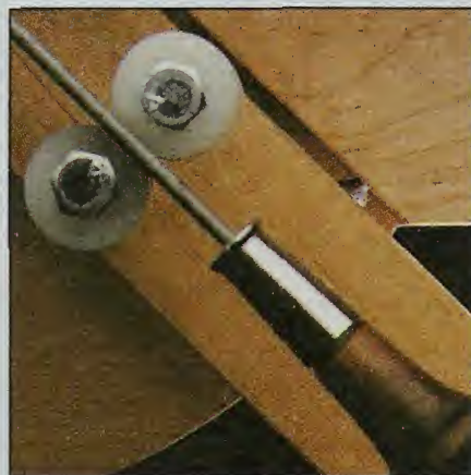
Step 2: Next, cut a test piece to check the accuracy. To fine tune the 45° angle, move the adjustment screw in or out until the angle is perfect.
