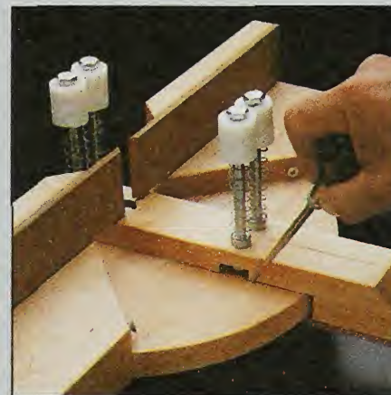
Step 3: To position the pivot arm for 90° cuts, repeat the process of rough positioning the arm and making trial cuts. Then scribe a line on the base.
