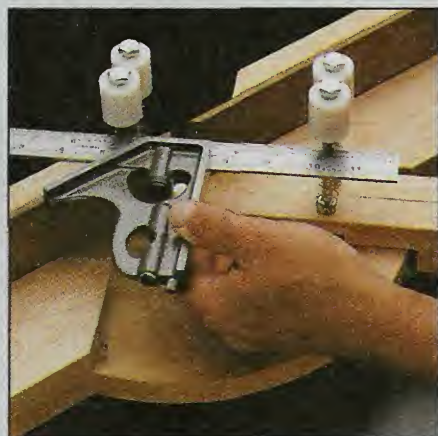
Step 1: Place the 45° face of a combination square against fence. Then pivot the arm so guide bolts touch the edge of the blade and lock arm in place.
