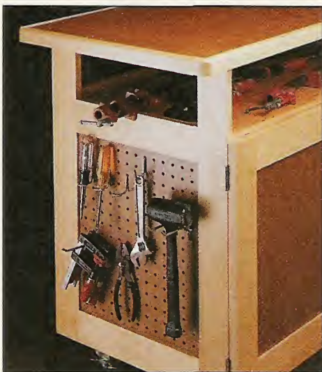
▲ Pegboard panels are a convenient way to keep tools and accessories handy. And an open shelf under the top is the perfect place for storing clamps.
