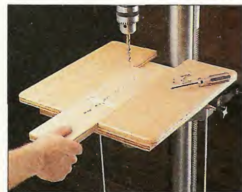
▲ When the insert gets chewed up after drilling many holes, just remove the old insert and screw on a new one.
