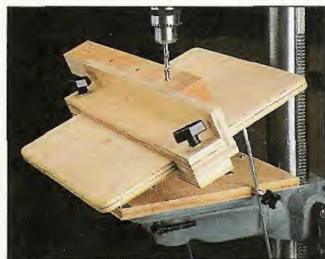
▲ Locking the fence on the top of the table helps hold the workpiece in place when drilling angled holes.
