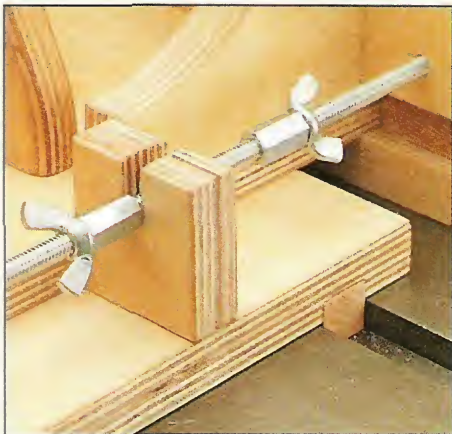
(A) Double-Stop System: This unique stop system lets you cut both cheeks of a tenon without flipping the workpiece.
