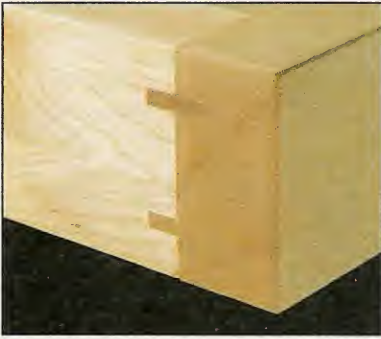
▲ The aprons are attached to the top with a spline and groove joint. These splines also lock the corners of the aprons together.
