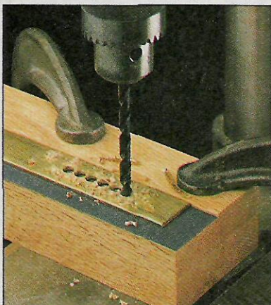
Cutting a slot in brass is as simple as drilling a series of non-overlapping holes (as shown), then filing the slot smooth.
