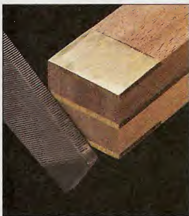
Shaping the ends of the handle is easy. You can use a smooth mill file (as shown), or a drum sander in a drill press.
