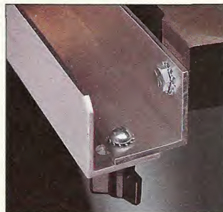
C. Adjustable Rail: The two-piece front rail is designed so you can adjust the angle of the fence to get a straight cut.
