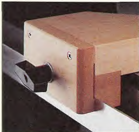
A. Fence Clamp: Built into this fence is a two-piece clamp that pinches the front rail and locks the fence in position.
