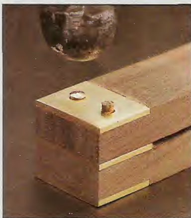
Rivets made from brass rod “draw” the handle pieces tightly together when the ends are peened over like a mushroom.
