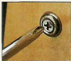
Finish washers prevent wood-screws from digging too deep into the plywood.
