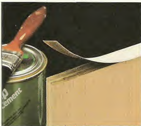
A. Glue-On Edging. Contact cement creates an “instant” bond between glue-on veneer edging and the plywood.
