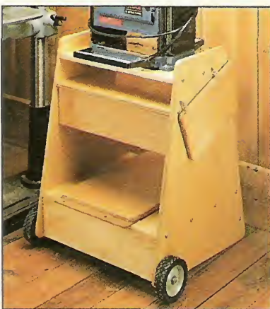
▲ The outfeed extension of the planer stand “knocks down” for moving and storage. The table lifts off and the “wings” fold back.
