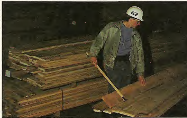
▲ The lumber grader checks each board as it comes off a pallet. He flips the board to look at both faces and then uses a set of lumber guidelines to assign a grade.
