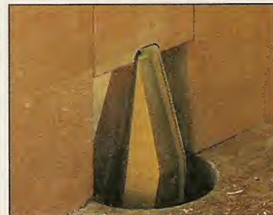
▲ To prevent chipout, a sliding insert forms a "zero-clearance" opening around the tip of the bit.
