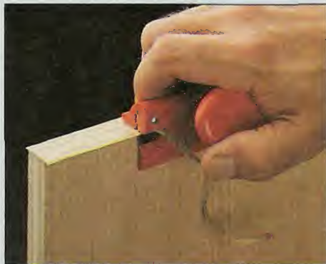
Single-Edge Trimmer. As a fence rides against the edge, the blade on this trimmer cuts the overhanging edge flush with the surface of the plywood.
