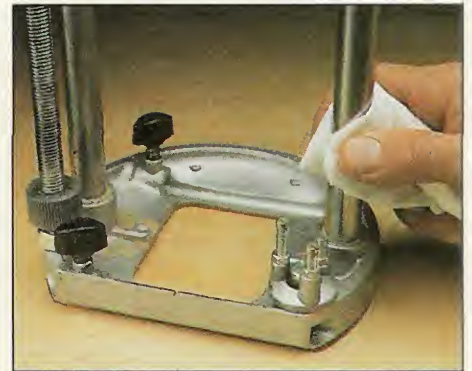
Plunge Tubes: Use a soft rag to clean the plunge tubes and rods. Then follow up the cleaning with a dry lubricant.
