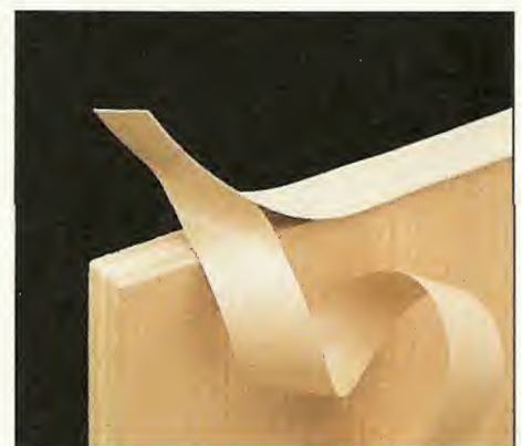
C. Veneer Tape. This is the easiest of the edgings to apply. Just peel off the backing and press the strip into place.
