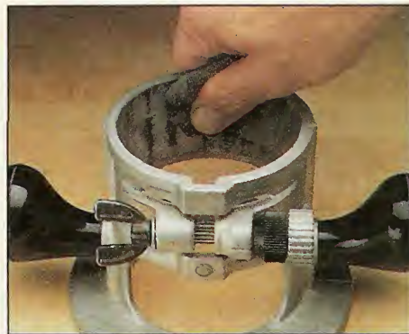
Pin and Groove: Steel wool works well to remove burrs and scratches that can form on the motor housing and base.
