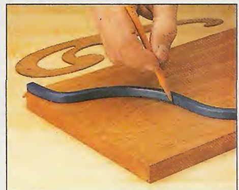
Curves: Flexible curves and French curves are handy for laying out or transferring graceful curves on a workpiece.
