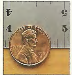
A penny is exactly \frac{3}{4} ". It's handy for quick measuring or laying out a \frac{3}{8} " radius on a corner.
