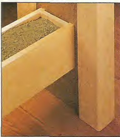
To add stability, a hollow wood beam is filled with sand. This anchors the stand and dampens the vibration of the lathe.
