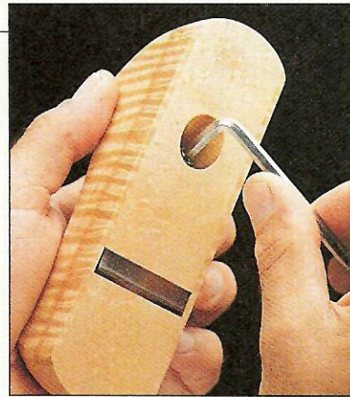
The blade is held in place by tightening the socket head cap screw with an Allen wrench.
