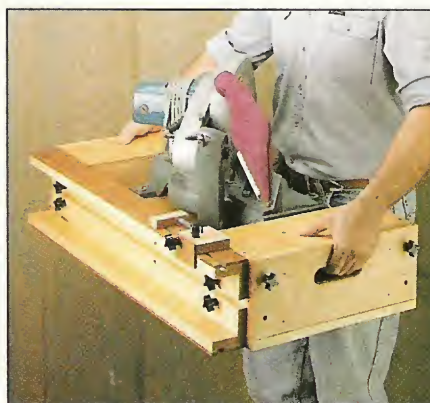
B. Portable: To make it easy to lift and carry the miter saw station, the wings have built-in handles.
