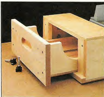
A. Wings: A pair of wings offer support to long stock and then "tuck" away inside the case for storage.
