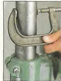
Use a C-clamp to measure the diameter of the drill press column.
