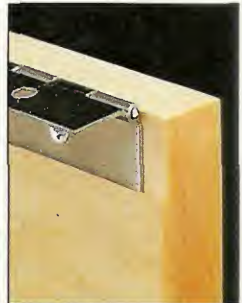
It's easy to install a piano hinge when you cut a shallow "alignment" rabbet for it to sit in.
