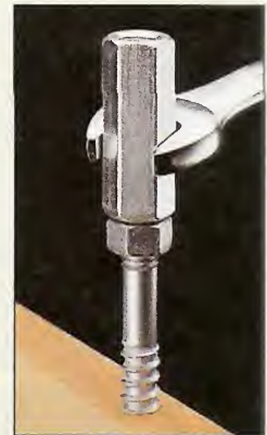
To protect the full length of the threads on a hanger bolt, I use a coupling nut. A "jam" nut prevents the coupling nut from turning.
