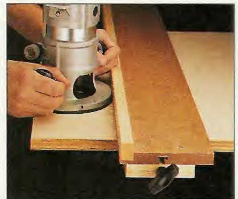
The fence doubles as a straightedge to guide the base of your router. Since the clamping system is beneath the guide, it won't get in the way of the motor housing.
