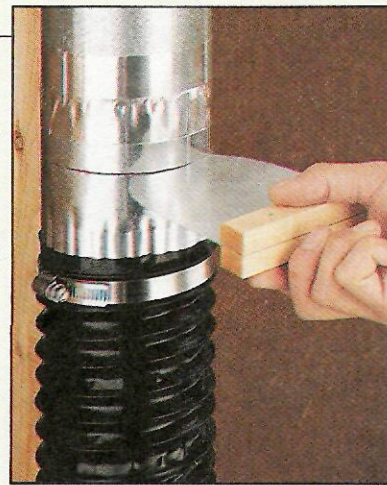
Sliding a shop-made blast gate in and out of a pipe turns the suction off (or on) at each tool.
