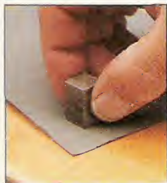
To smooth a rough metal guide block, just rub it on a piece of silicon-carbide sandpaper.
