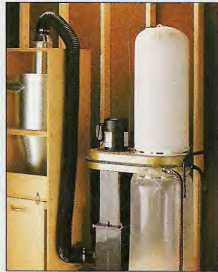
To connect a portable dust collector, run a flexible hose from the inlet of the vacuum to the cyclone.
