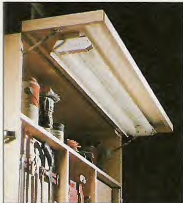
▲ Optional Light. The flip-up door is sized to accept a standard four foot shop light.
