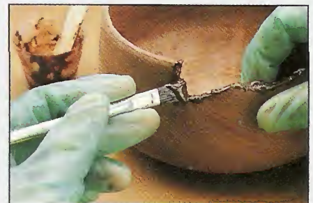
Step 3: Apply the thickened mixture to one surface only. Then bring the parts together and allow to cure.
