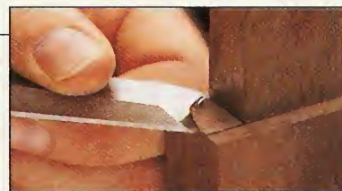
An underhand grip helps control the cut when paring the "step" off a tenon.
