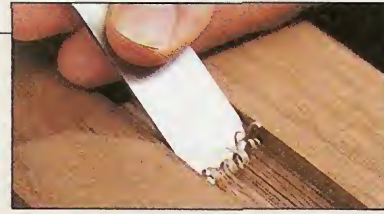
Use the chisel with the bevel face down to keep from cutting too deeply into the bottom of a groove.
