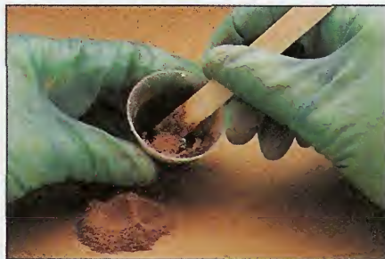
Step 2: Now you can add filler to the remaining mixture. Keep adding filler until desired consistency is reached.
