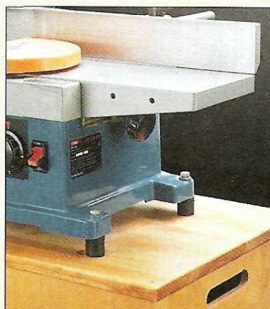
▲ Isolation Mounts. Hard rubber cylinders "isolate" the vibration set up by the motor on a tool.
