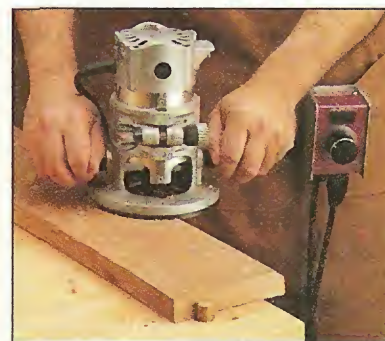
▲ Speed Control. To reduce the RPM's (and noise) of a fixed speed router, use a speed control unit.
