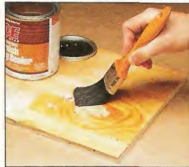
Step 2. To help the contact cement stick, seal the surface with a thin coat of sanding sealer.
