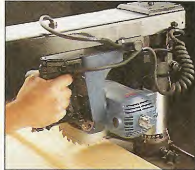
▲ Universal Motor. Because it operates at high speed, a tool with a universal motor runs louder.
