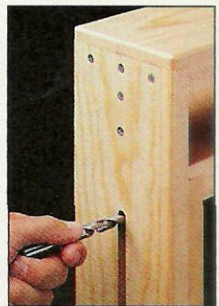
With the support pushed all the way down, use a brad point drill bit to locate the hole for each hex bolt.
