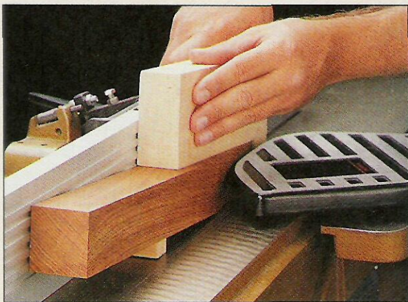
▲ To cut a short taper, a block of wood raises the untapered end of the workpiece off the jointer while the opposite end rides across the cutterhead.
