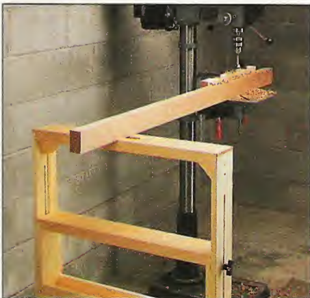
A. Work Support. This sawhorse can support a long workpiece when working at the drill press or band saw.
