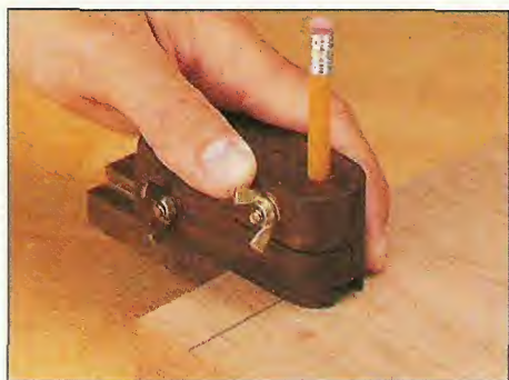
A. Marking Gauge. This marking gauge fits in the palm of your hand (or the pocket of your shop apron) and uses a pencil to produce highly visible lines.
