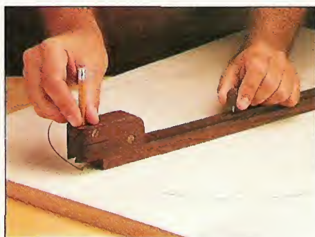
B. Beam Compass. When used as a beam compass, the layout tool allows you to lay out just about any size arc or circle you'll need.
