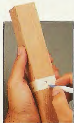
Marking numbers on the tape provides an easy way to keep track of the cutting sequence.
