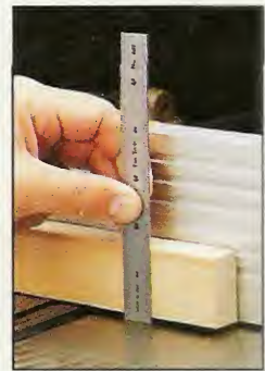
To determine the depth of cut, measure the gap between the infeed table and a straight stick laid across the outfeed table.
