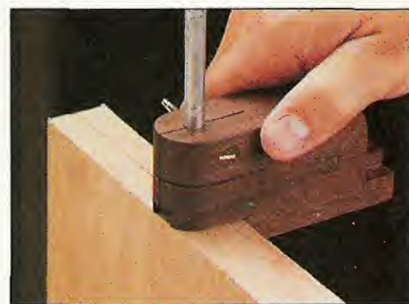
C. Cutting Gauge. Using the leftover material, you can make a second head to hold an X-Acto knife. This will allow you to score layout lines.
