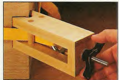
▲ Now fit the jaws of the clamp on a corner of the project, reposition the strap (if necessary), and tighten the wing nut.
