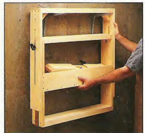
C. Compact Storage. When it’s not in use, you can knock down the sawhorse and store the feet in the tray.
