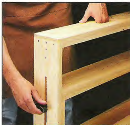
B. Adjustable Height. To adjust the height, just loosen the knobs on the sides and raise or lower the sawhorse.
