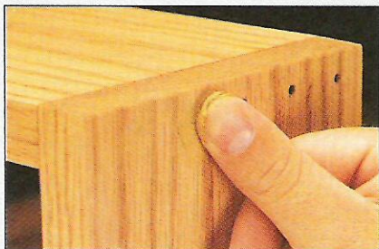
Non-Hardening. This type of filler is applied directly to a stained project. The finish can follow immediately.
