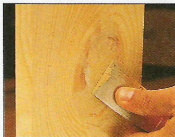
Hardening. A hardening filler is used on projects with a natural or painted finish. After
