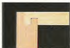
Bit is correct height.
