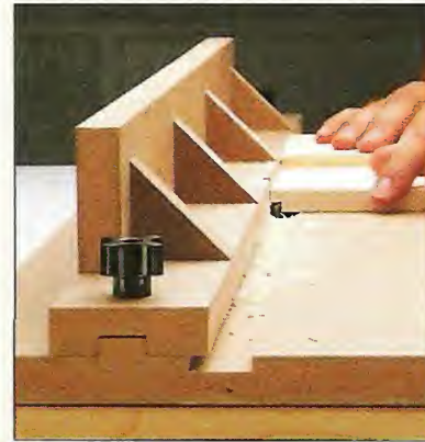
Back. Because the groove that fits over the key is offset, the back of the fence allows you to cut a rabbet on the end of a workpiece.
