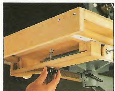
C. Fence Brake. Once the fence is adjusted where you want it, lock it in place by tightening the knob on the brake.
