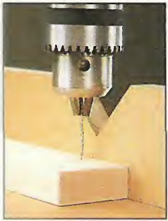
To allow the drill press chuck to clear the fence when using short or small bits, I cut a V-notch in the center of the fence.
