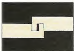
Fence is too close to bit.
