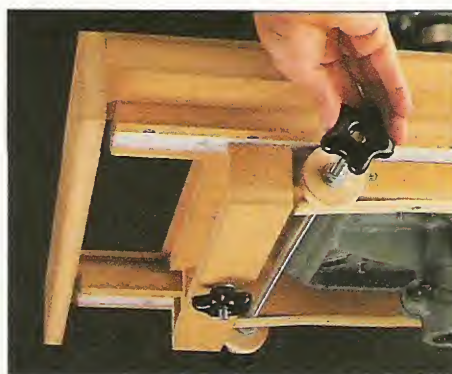
B. Micro Adjuster. A mechanism under the table allows you to micro-adjust the fence to fine tune the position.
