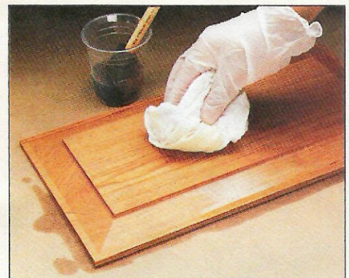
B. Remove Excess. Now wipe off all the excess oil so the wood looks “dry.” When the oil cures, apply additional thin coats until you get the desired sheen.
