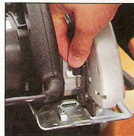
Depth Adjustment. The plastic knob on the Quantum (left) provides a more comfortable grip than the wing nut on the B&D (center). But neither are knuckle-busters like the depth adjustment lever on the Skil (right).
