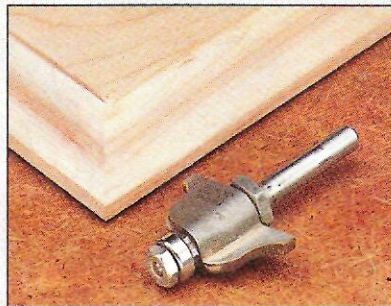
▲ Ball-Bearing Pilot. But when a ball bearing pilot rides along the edge, the bit spins freely inside and leaves a clean edge.
