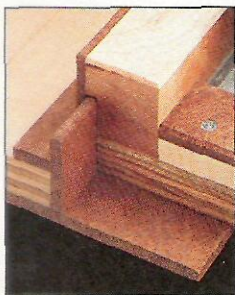
To ensure straight, accurate cuts, a hanger on the carriage hooks over the fence on the cutting guide.
