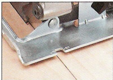
Indicator. Unlike the fixed notch on the Skil saw (left) that marks the path of the blade, the indica-
