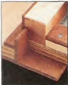
To ensure straight, accurate cuts, a hanger on the carriage hooks over the fence on the cutting guide.
