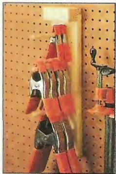
To save space, this spring clamp hanger is designed to "nest" your clamps.
