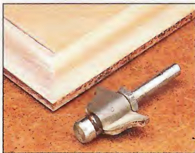
▲ Solid Pilot. As a solid pilot rubs against the edge of the workpiece during a cut, it tends to burn or burnish the surface.
