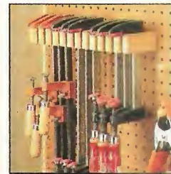
To hang a bar clamp on this hanger, just slide down the bottom jaw and slip the clamp in place.
