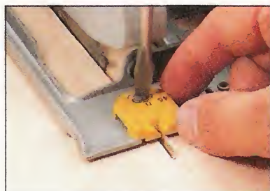
tor on the Quantum (right) can be adjusted if you use blades that vary in thickness.
