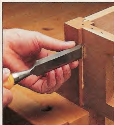
E. Remove Glue. After you've assembled the project, scrape off the “skinned over” glue with a chisel.
