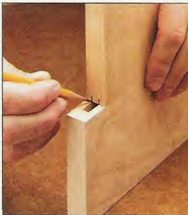
Thickness. To establish the thickness of the tenon, draw lines just inside the walls of the mortise.
