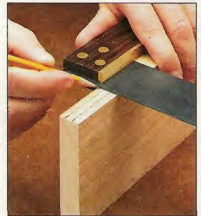
Length. Use a try square to lay out the shoulders and determine the length of the tenon.
