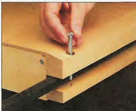
B. Removal. The outfeed table can be quickly and easily removed from the saw by pulling two quick-release pins.
