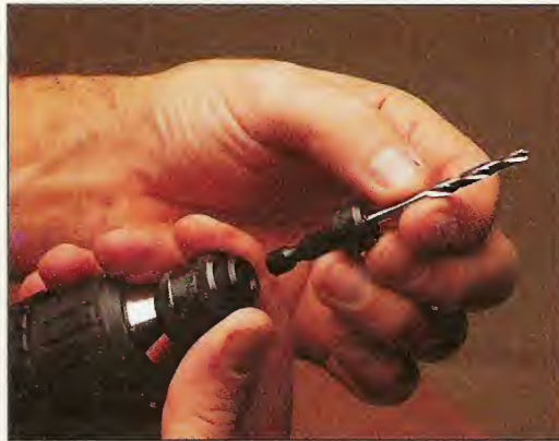
Adapter. One quick-change bit system uses an adapter to hold a hex shanked drill or driver bit. To insert a bit, just pull back on the collar.
