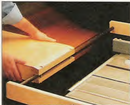
A. Position. You can position the outfeed table anywhere across the back of the table saw — for any size workpiece.
