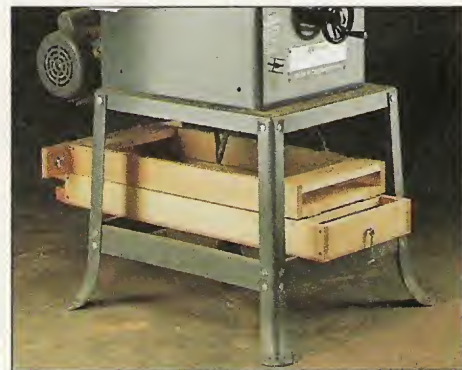
C. Storage. When you’re through using the outfeed table you can fold it up for compact, space-saving storage.
