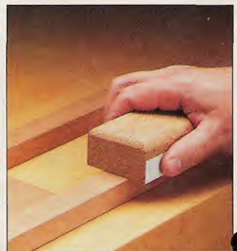
C. Hand Sanding. But on a narrow workpiece, a sanding block ensures a crisp corner and a flat surface.
