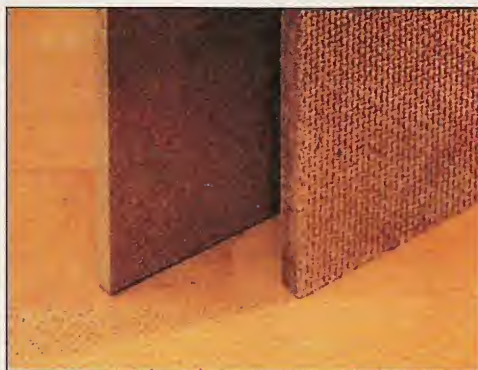
B. Textured Back. This "waffle" imprint is typical of what you'll find on hardboard that's smooth on one side only.
