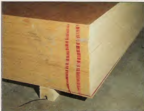
A. Class Markings. Two red stripes indicate service-tempered hardboard. One green stripe indicates standard hardboard.
