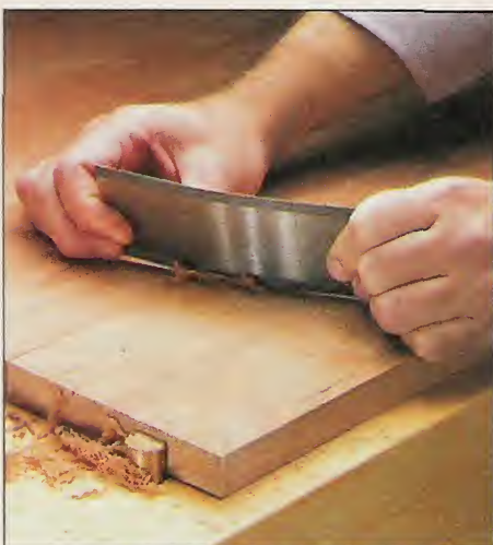
A. Scraper. Use a scraper to remove any tool marks or ridges. Skew the scraper at an angle for the best cut.
