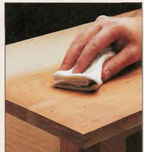
F. Mineral Spirits. Wiping down the surface with a rag soaked in mineral spirits reveals stray glue smudges.
