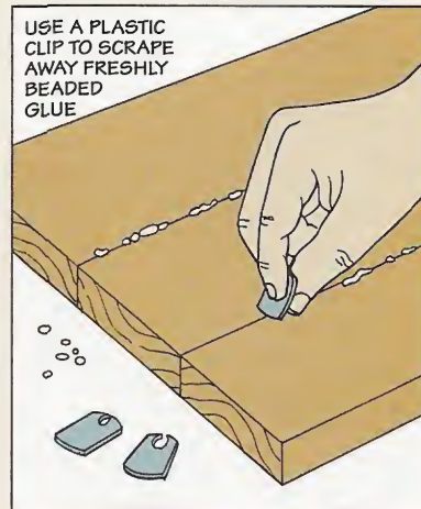
Glue Scraper. Use a plastic clip from a bread bag to scrape away skinned-over beads of glue from a flat surface.
