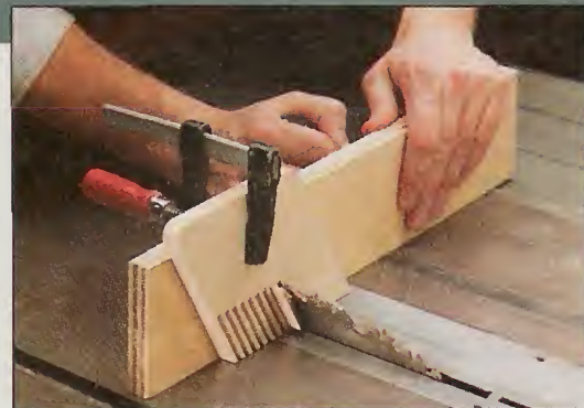
Perfect Kerfs. The index pin makes it easy to cut evenly-spaced kerfs. Just index the workpiece on the pin between each pass.
