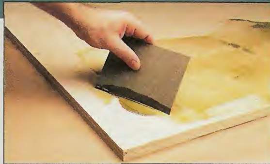
Trowel. The key to a good bond when working with contact cement is to spread the cement evenly. To do this, I use a small, hand-size piece of plastic laminate as a trowel.
