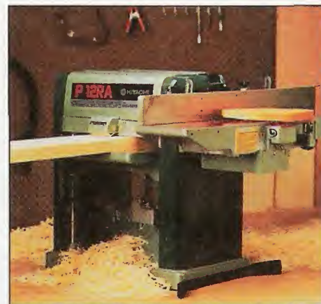
▲ This Hitachi P12RA planer/jointer combines a 12" thickness planer with a 6" edge jointer. A combination tool like this takes up less space than two similar, separate bench-top power tools. (Hitachi Power Tools: 800-362-7297)
