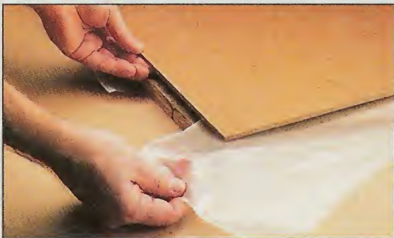
Non-Stick Barrier. Waxed paper between workpieces gives you a chance to make last minute adjustments. Once the pieces are aligned, pull out the paper and apply pressure.
