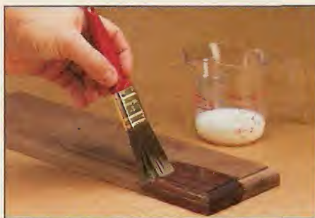
B. Brush. A synthetic bristle brush (nylon or polyester) helps lay down a smooth coat of finish on small pieces.
