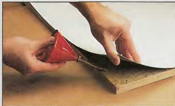
Emergency Release. In the event of a disaster, you can separate the two workpieces by flowing a liberal amount of lacquer thinner between them and gently peeling off one of the layers.
