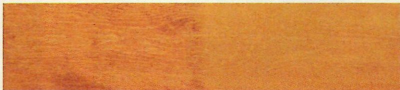
A. Wood Conditioner. Applying an oil-based stain directly to this piece of pine creates a series of light and dark blotches (left). But using a wood conditioner first helps even out the color (right).
