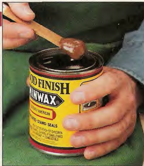
▲ The thick sludge that settles to the bottom of a can of oil-based stain is formed by small colored particles or pigments.
