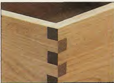
Perfect Fit. On a perfect-fitting joint, the pins are flush with the sides, and there are no gaps.
