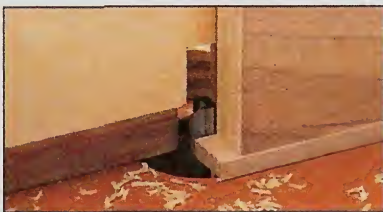
▲ To trim the edging flush, a rabbet provides a recess for the lip that sticks up above the surface.
