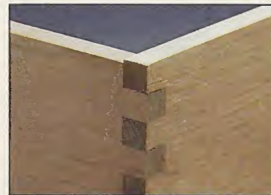
Offset. An offset can be caused by not having a workpiece fully seated on the index pin or the jig.
