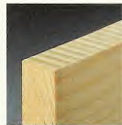
To prevent a "scalloped" edge, try slowing down your feed rate.
