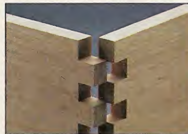
Too Tight. If the pins won't fit in the slots, the index pin is set too far away from the router bit.
