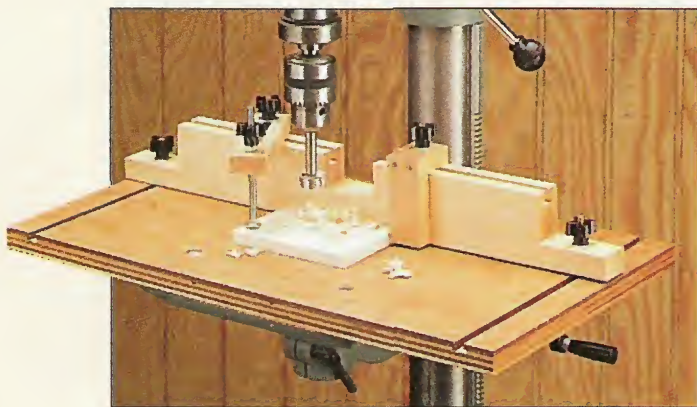
Accurate Drilling. The fence on this drill press table uses a stop block and a hold-down for clamping and accurately positioning a workpiece.
