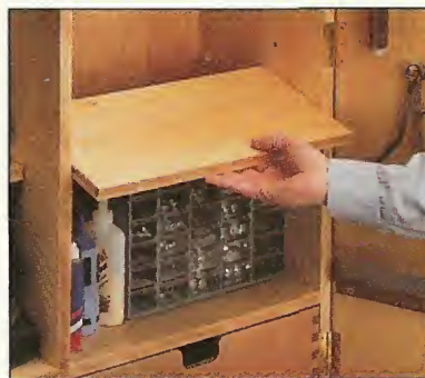
B. Shelves. Adjustable shelves provide additional storage. And they stay put when removing a tool.
