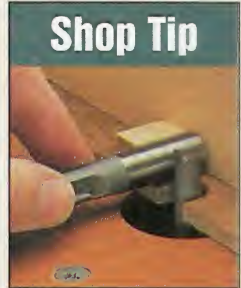
Shop Tip The shank of a router bit makes a handy gauge to set up pin spacing.
