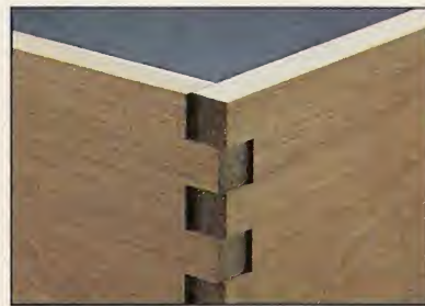
Short Pins. If the router bit is set too shallow, you'll end up with pins that are too short.
