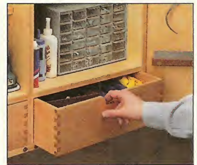
C. Drawers. Sturdy drawers held together with box joints are used to store accessories and supplies.
