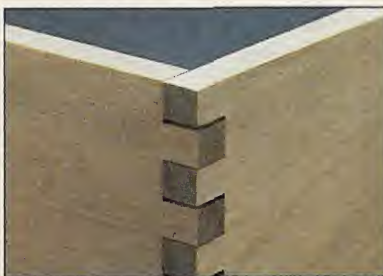
Gap. A gap between each pin and slot is caused by an index pin that's too close to the bit.
