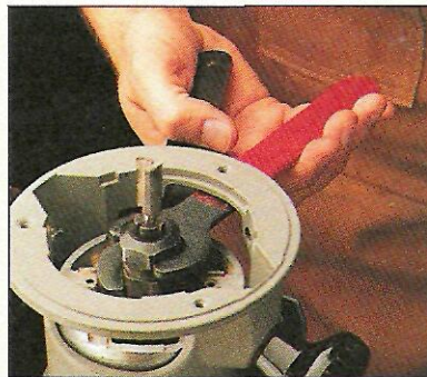
Loosen Collet. To loosen a collet, reposition the wrenches and just squeeze them together.
