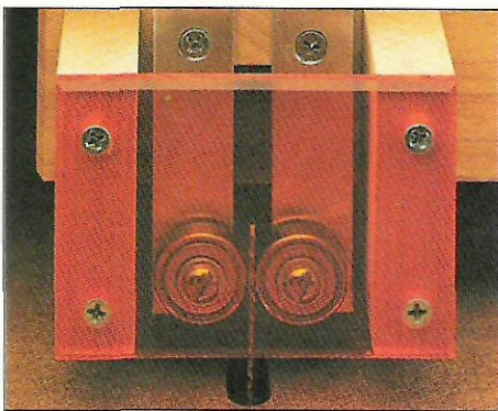
A. Guide System. To ensure a perfectly square cut, a pair of bearings prevents the blade from moving side to side.
