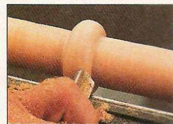
▲ A simple bead is formed by rolling the gouge over on its side.
