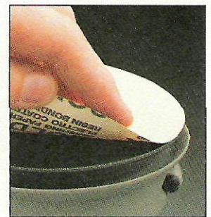
Pads. A hook & loop system (left) makes it quicker and easier to change sanding discs than a pad that uses pressure sensitive adhesive discs (right).
