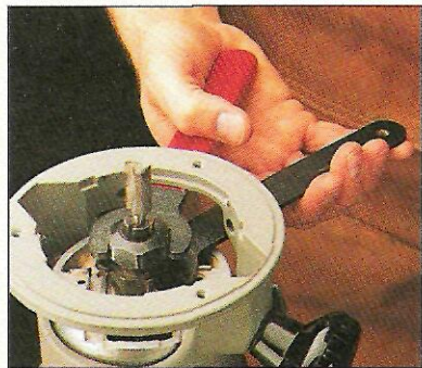
Tighten Collet. A single grip and a squeeze are all it takes to tighten a bit in a collet nut.
