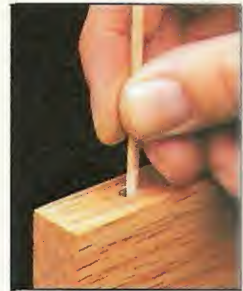
To quickly coat a hole with glue, stir the glue around with a dowel.
