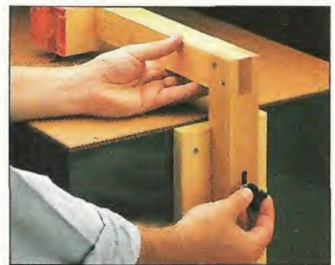
C. Adjustable Arm. The arm that supports the guide system and hold-down adjusts for different thicknesses of stock.
