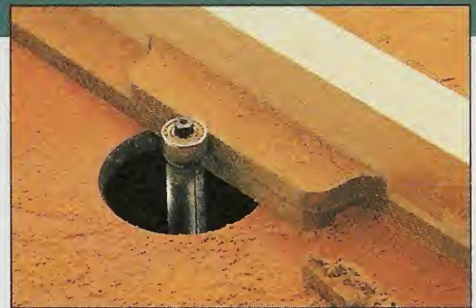
Identical Parts. A quick way to produce identical parts is to make a template and use it as a pattern for a flush trim bit to follow.
