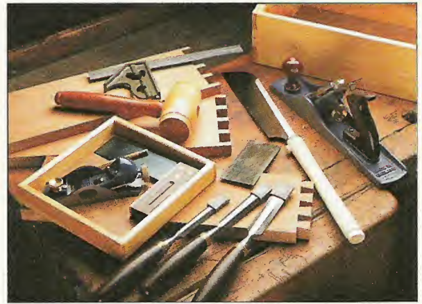
Hand Tools. A chisel set, a few hand planes, and a square or two are just a few of the hand tools that should be in every woodworking shop.
