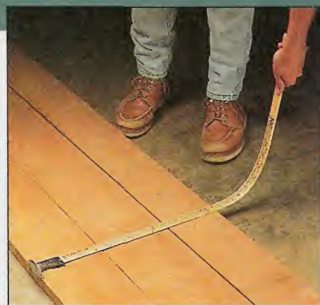
Lumber Scale. A lumber scale allows you to quickly figure board footage. For your nearest dealer call the Conway-Cleveland Corporation (616-458-0056).
