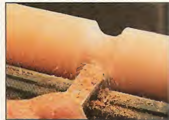
▲ To create a clean, crisp cove, make a scooping cut with the gouge.
