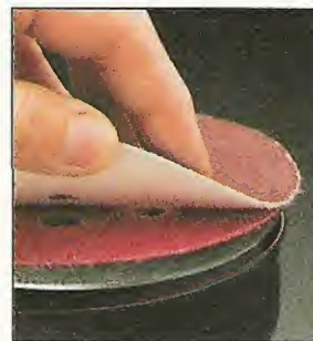
Pads. A hook & loop system (left) makes it quicker and easier to change sanding discs than a pad that uses pressure sensitive adhesive discs (right).
