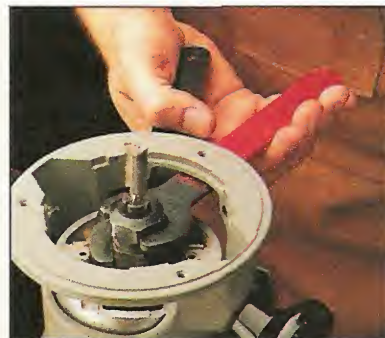
Loosen Collet. To loosen a collet, reposition the wrenches and just squeeze them together.
