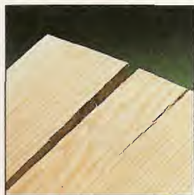
Physical Defects. Lumber with physical defects such as checking (left), planer snipe (center), and chipout (right) can be used. But if there are other boards to pick from, I'll generally pass on those with these defects.
