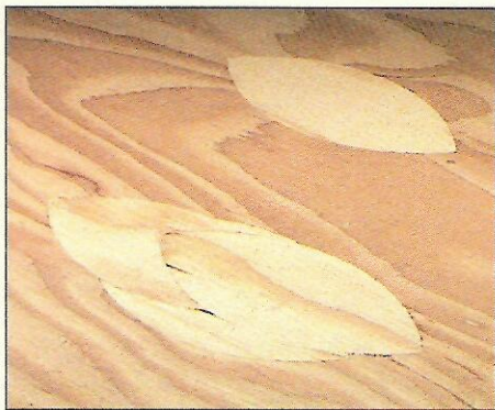
A. Patches. Large knots on A and B grades of softwood plywood are usually replaced with football-shaped patches.
