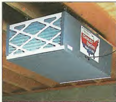
Suspended Filter. If floor space is a premium, consider a filter unit that can be suspended overhead.
