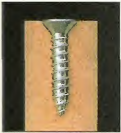
To avoid splitting MDF, drill pilot holes and use a screw with a straight shank.
