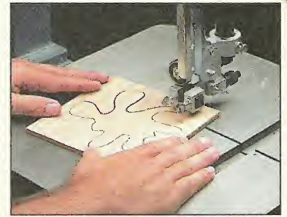
Scroll Cuts. And cutting tight curves with an 1/8" blade put the saw's guide system to the test.
