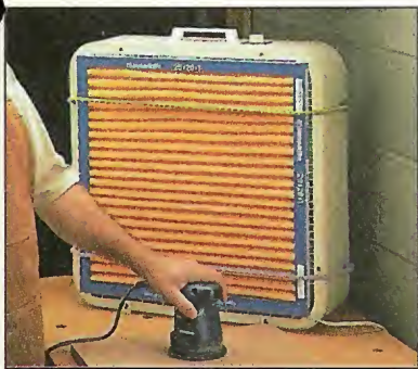
Fan Filter. One way to reduce air-borne dust in the shop is to attach a pleated filter to a household fan.
