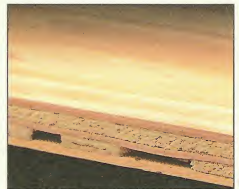
C. Voids. In addition to the face veneers, you can get a feel for the quality of the plywood by checking for voids.
