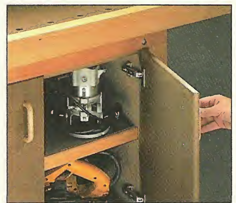
C. Cabinet. The cabinet is a convenient place to store hand tools. It also adds extra mass to the workbench.
