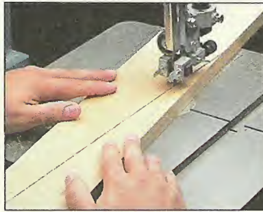
Shapes. Cutting irregular shapes and curves with a 1/4" blade showed how well the saw held to a line.
