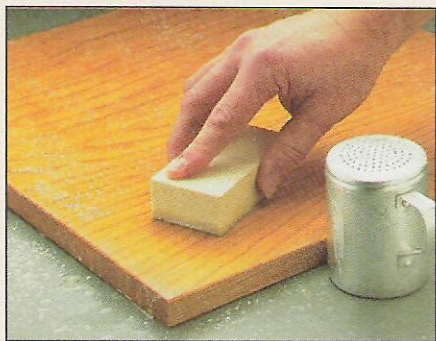
Step 3. Now rub the finish with pumice and a felt pad to produce a satin sheen. Rottenstone creates a gloss finish.
