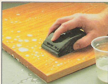
Step 1. With soapy water as a lubricant, use Wet-or-Dry sandpaper and a rubber block to sand the finish flat.
