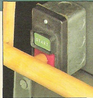
Push-Button. To build the knee bar, you'll need a pushbutton switch like this.
