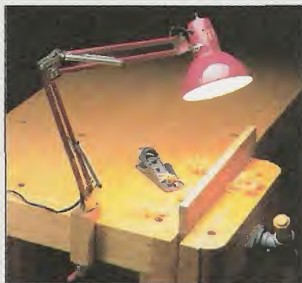
Bench. Clamping a shop-made bracket to the edge of your bench allows you to direct light from an ordinary student lamp exactly where you want it.
