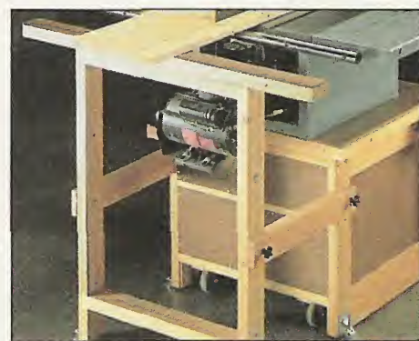
C. Outfeed. To make cutting large workpieces more manageable, an outfeed support attaches to the stand.
