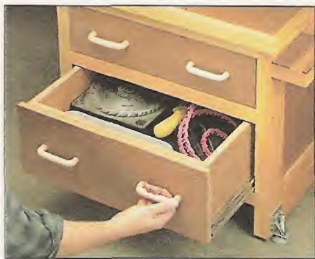
A. Storage. Saw blades and accessories are stored in a large drawer. And brackets hold the rip fence and miter gauge.
