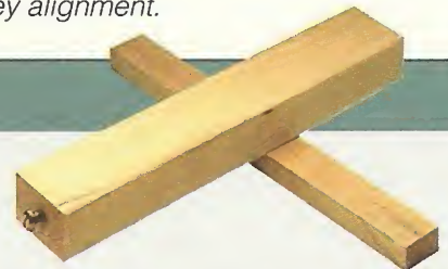
▲ A straightedge is a quick and easy way to check the arbor and motor pulley alignment.
