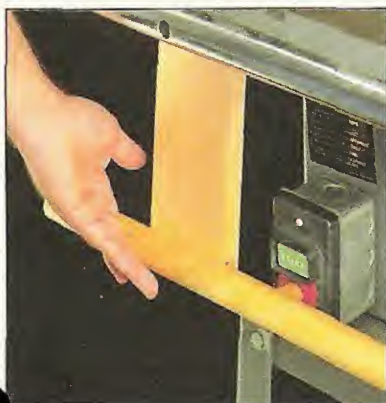
Hand Operated. The shut-off bar is designed to be knee operated, but you can also use your hand.
