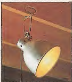
Utility Lights. A clip-on utility light (left) or a lamp with a magnetic base (right) help fill in shadows when you’re doing close-up work.
