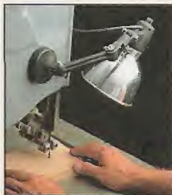
Utility Lights. A clip-on utility light (left) or a lamp with a magnetic base (right) help fill in shadows when you’re doing close-up work.
