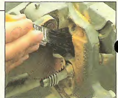
It may be necessary to soak pitch and resin build-up with solvent to help break it free.
