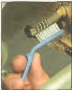
To get at hard to reach places, heat the handle of a toothbrush and bend it at an angle.
