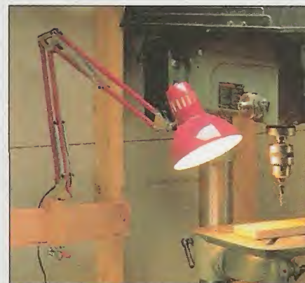
Wall. To illuminate close-up work at a power tool, clamp the bracket to a wall-mounted block ripped to the same width as the thickness of the bench.
