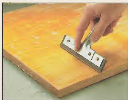
Step 2. Remove the slurry with a squeegee and check for a dull, uniform sheen. Shiny areas indicate low spots.
