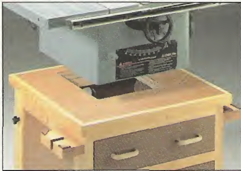
▲ A built-up top with a hole cut in it allows sawdust to fall through. It also provides a sturdy platform to mount the table saw.
