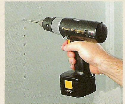
C. Clutch. Screwing sheetrock to wall studs gave us a feel for how well we could fine tune the clutch.
