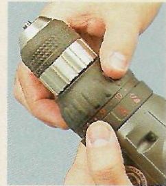
A separate lockout ring on the Black & Decker allows you to switch quickly from "drive" to "drill" mode.
