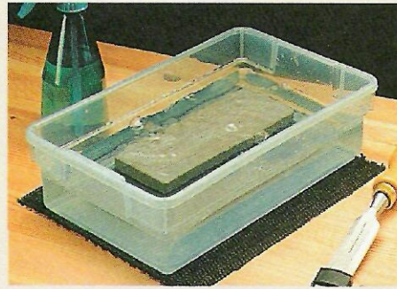
◀ Soak Stone. Put the stone in a container of clean water. It's ready to use when bubbles stop rising to the surface (about five minutes).
