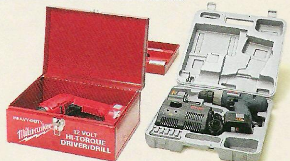
Cases. A metal case with a continuous hinge (like the one that comes with the Milwaukee at left) is sturdier than the Ryobi's plastic case with its "web" hinge (right).
