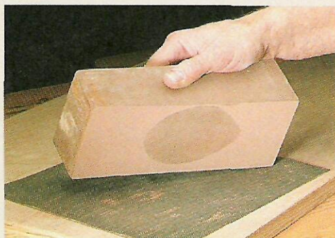
Truing a Waterstone. The dark areas and "dished" surface of this stone are indications that it needs flattening.
