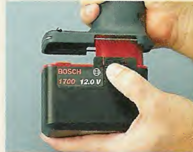
Batteries. A metal clip on the Porter Cable (left), Skil, and Makita holds the batteries securely in place. But it's not as handy as the snap-in batteries on the rest of the drills. (Bosch is shown at right.)
