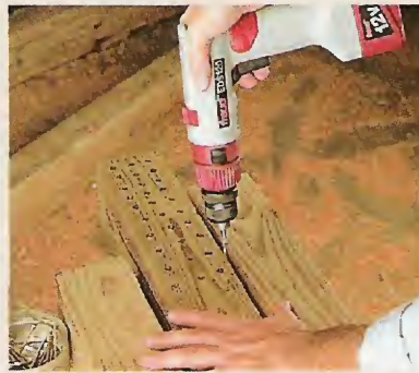
B. Driving. And we compared their performance when driving 3" deck screws in pressure treated lumber.
