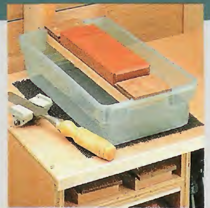
▲ Spanning a plastic container filled with water, a simple holder anchors the sharpening stone.
