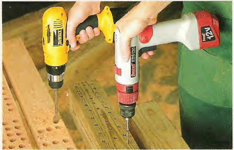
▲ If you're in the market for a cordless driver/drill, there are two body designs to choose from — a T-handle (left) and a pistol grip (right). Either way, these 12-volt models have plenty of power.
