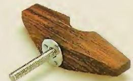
You can make a threaded stud by epoxying a cutoff bolt in the T-nut.
