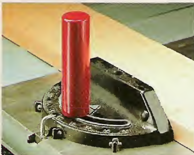
▲ This tall dowel provides a more secure grip on the miter gauge than the handle it replaces.
