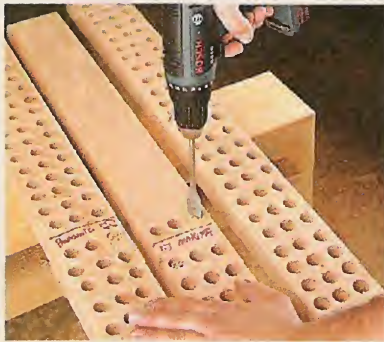
A. Drilling. To test how much "gas" these drills had, we drilled 3/4"-diameter holes in Douglas fir.
