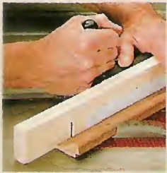
To prevent a workpiece from "creeping" during a cut, attach sandpaper to your auxiliary fence or miter gauge head.
