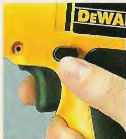
Forward/Reverse. It's easy to operate the forward/reverse switch when it's on the body of the drill
