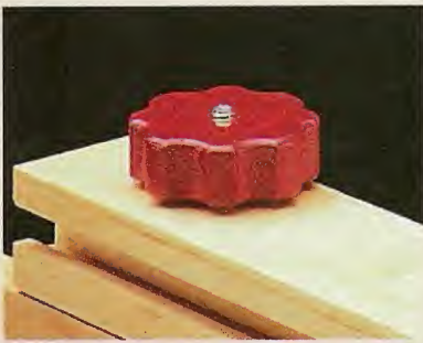
▲ The scalloped edges on this star knob make it ideal for applying pressure comfortably.
