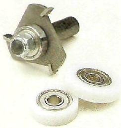
A slot cutter bit makes quick work of routing a groove for a spline. And different size bearings let you adjust the depth of cut.
