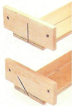
With two inserts, you can use one for 90° cuts (top) and the other for 45° cuts (bottom).
