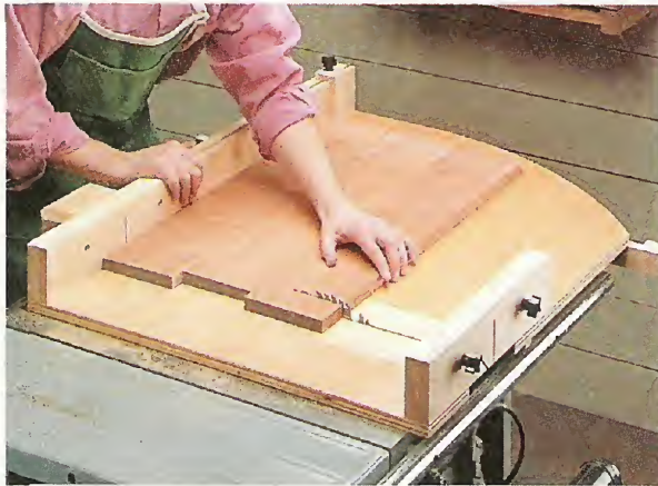
Wide Panels. To make accurate crosscuts on panels up to 24" wide, this sliding cutoff table combines a large plywood platform with a long fixed fence.
