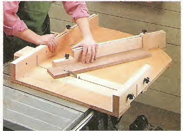
Angled Cuts. By attaching an adjustable fence that pivots around the curved end of the sliding table, you can make angled cuts as well.
