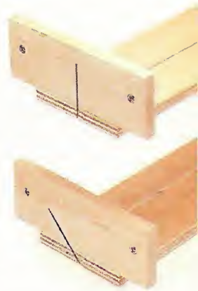
With two inserts, you can use one for 90° cuts (top) and the other for 45° cuts (bottom).
