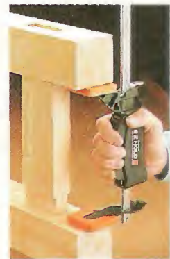
Simply reversing the jaws on the E-Z Hold clamp allows you to use it as a spreader.
