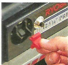
Unlike the loose safety key on the Makita (top), the other planers use a plastic tab that snaps onto the switch (bottom).
