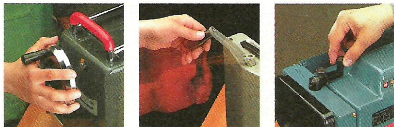
Depth of Cut Adjusters. The handwheel on the Sears (left) and a folding crank on the Delta (center) are handy to use. But the crank on the Makita (right) has a lock knob that makes it a knuckle-buster.
