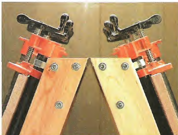
B. Two Work Surfaces. Each side of the glue-up station is designed to hold pipe clamps. So you can glue up several panels at once.
