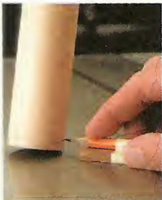
Using a pencil and a scrap of hard-board, mark a line around the bottom of each leg.
