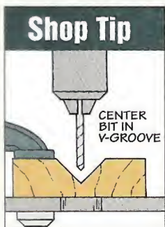
A small drill bit makes it easy to center the V-shaped groove.
