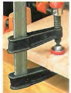
Tightening a clamp across the end of a joint line draws the surface of the boards flush.
