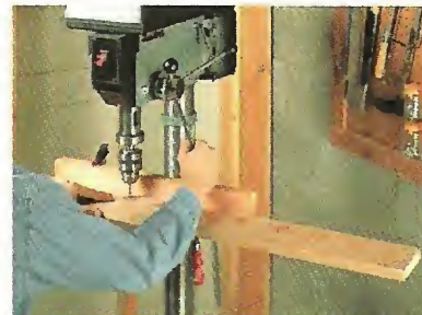
D. Corners. Even with this drill press tucked in a corner, you can still work with long workpieces.
