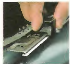
A feeler gauge is a clumsy way to set the blades (top). But spring-loaded blades that snap to a bar (center) and a magnet (bottom) that sets the blade on a backing plate are easier to use.
