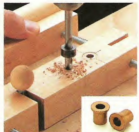
C. Guide Holes. To reduce wear from repeated drilling, each guide hole is lined with a pair of bronze bushings.
