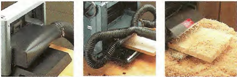
Dust Hoods. A single port on Delta's dust hood (left) doesn't clog up during a heavy cut like the dual ports on the Jet (center). With no dust hood, the Sears (right) throws chips everywhere.
