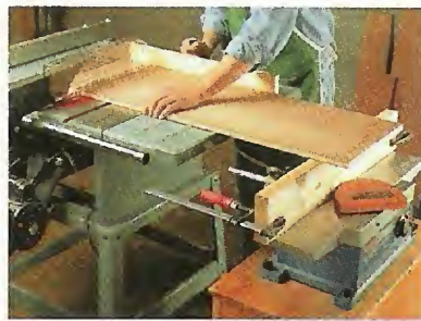
A. Support. A board clamped to the fence of the jointer provides support for a long workpiece.
