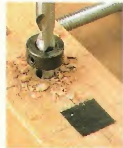
To make sure you drill in the same guide hole each time, tape over the one you're not using.
