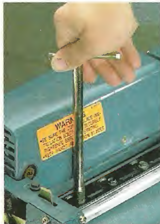
Hand Position. Changing blades on the planers that use a gib system (above) puts your hand right in line with the cutting edge. But you don't run the risk of a nasty gash with the Makita's T-handle and backing plate (side).
