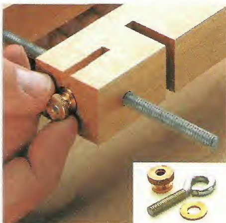
A. Locking System. Tightening a knurled nut pulls an eye bolt tight against a threaded rod to lock in the adjustment.
