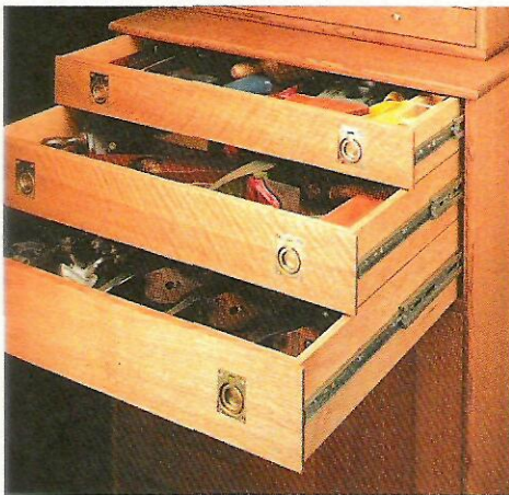
A. Drawers. To provide easy access, the three drawers in the rolling cabinet are mounted on full-extension slides.
