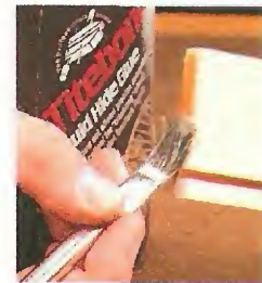
To provide more working time when gluing up the facing strips, I used hide glue.
