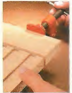
Cutting stopped dadoes is easy. Just cut the front edge off the panel. Then cut a series of through dadoes, and glue the front edge back in place.
