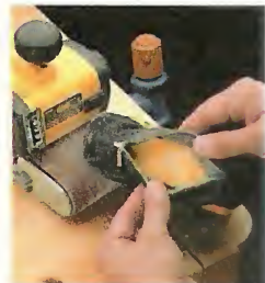
Dust Bags. Sliding a clip on and off when emptying a dust bag (top) isn't as handy as a zipper (center). But the zipper on the DeWalt (bottom) has a plastic support that makes the bag hard to empty.
