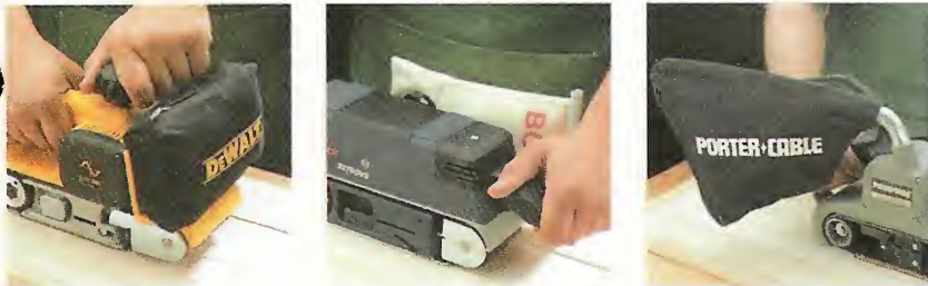
Dust Collection. The dust bag on the DeWalt (left) is small and out of the way. But it doesn't collect as much dust as the side-mounted bag on the Bosch (center) and the Porter Cable's rear-mounted bag (right).
