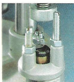
Turrets. The “stops” on the turrets that establish the depth of cut can either be fixed (top) or adjustable (bottom). Both types work equally well.
