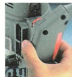
Plunge Lock. The plunge lock switch on the Sears (left) and the lever on the Makita (center) are easy to use. But you have to unlock the lever on the Porter Cable (right) to make a cut — and that's a nuisance.
