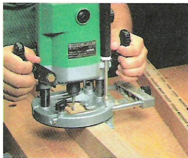
Mortises. To test plunge operation for smoothness and accuracy, we routed a series of mortises.
