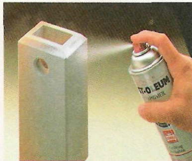
Step 2. Then apply a primer to provide a base for the paint and keep it from discoloring.
