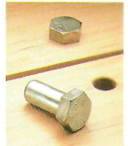
To make a simple bench dog, cut the threads off a bolt, and grind the sides of the head at a slight angle.
