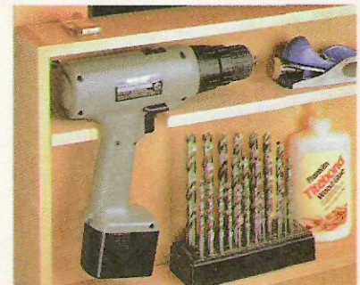
▲ To make a convenient holder for a cordless drill, just cut a simple notch in one of the shelves to fit the handle.
