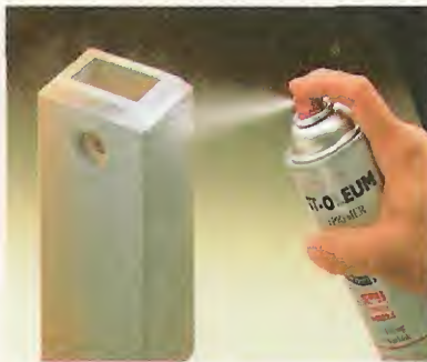
Step 2. Then apply a primer to provide a base for the paint and keep it from discoloring.
