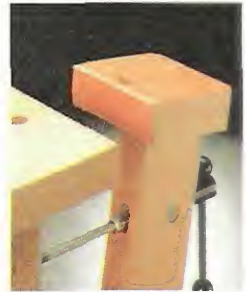
To hold carving blocks securely in place, you can glue leather strips to each clamping surface.
