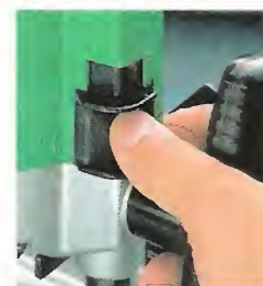
Switches. A trigger switch that's built into the handle (top) is handier to use than a toggle switch (center) or a slide switch (bottom).
