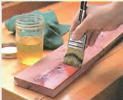
Sealer. Applying a two-pound cut of shellac to wood that has a lot of knots will seal in resins or sap that can bleed through and ruin a finish.
