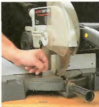
A. Set 0° Stop. After adjusting the 0° stop so it contacts a casting on the arm, align the indicator to the 0° mark on the bevel scale.
