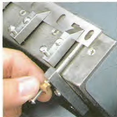
A. Stop. A micro-adjustable stop lets you fine tune the position of the knife. And a set of hold-downs keeps it securely in place.
