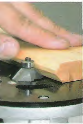
Chamfer Gauge. A scrap block with pre-cut chamfers makes it easy to set the height of the chamfer bit.
