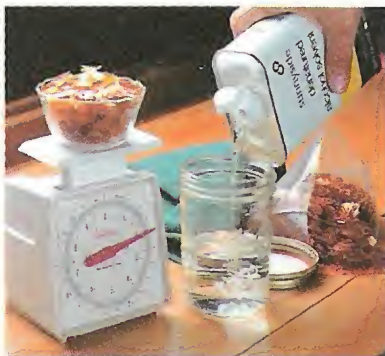
A. Cut. Weigh the flakes of shellac and measure out the alcohol to determine the correct "cut."
