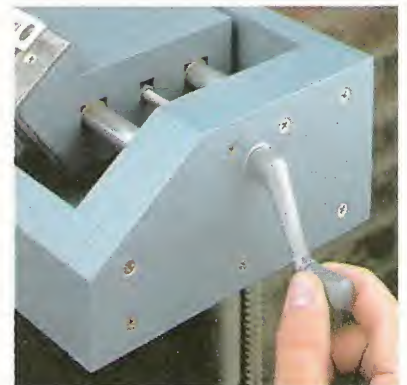
B. Crank. Turning a simple crank moves the carriage that holds the knife (or plane iron) back and forth under the grinding stone.
