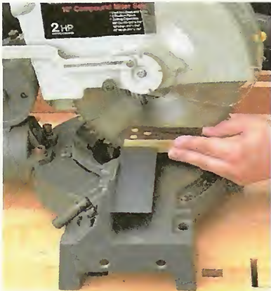
A. Adjust Turntable. After loosening two bolts on the bottom of the saw, adjust the turntable so the blade is square to the fence.
