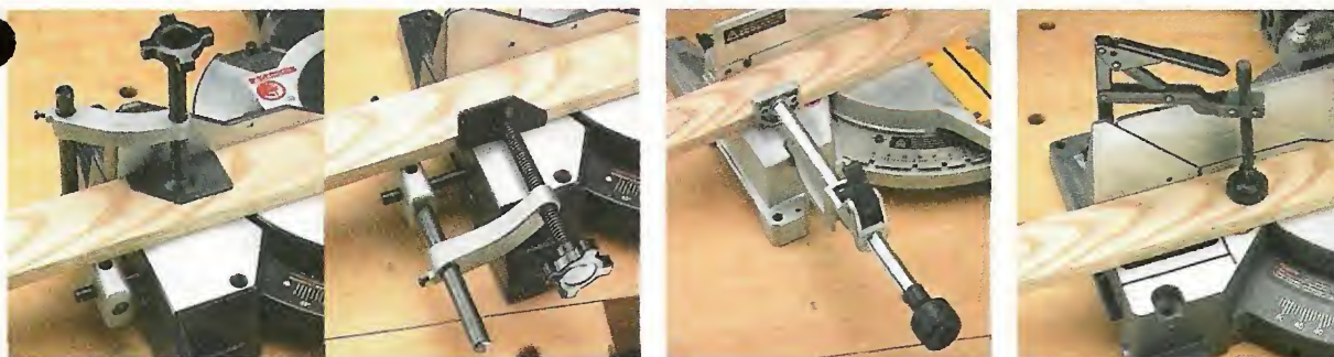
Hold-Downs. The hold-down on the Sears can be used to clamp work down against the saw table (left) or against the fence (left center). So it has a wider range of uses than the DeWalt (right center) that holds work against the fence only, or the Skil (right) that only applies pressure downward.
