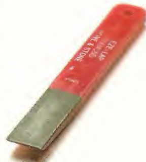
Use a fine diamond hone to remove the burr and add a secondary bevel to the edge of the knife.
