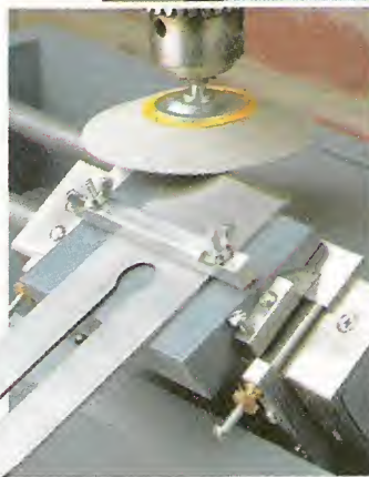
Double Duty. It's easy to get razor sharp edges on your jointer knives (top) or plane irons (left). Just turn the crank on this simple jig.
