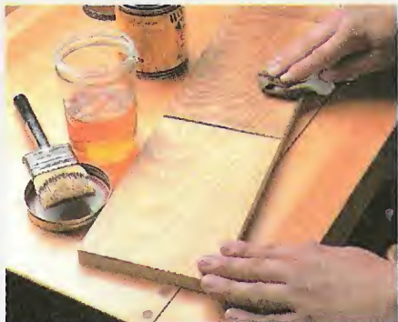
Conditioner. To help prevent blotching when staining softwoods, use a half-pound cut of shellac as a conditioner before you stain.
