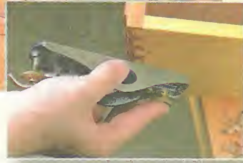
▲ Using his low-angle Record block plane, Steve Curtis (our shop manager) trims the pins of a dovetailed drawer.
