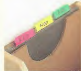
Using index tabs to separate different grits of sandpaper lets you find the sheet you need at a glance.
