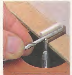
An 1/8" drill bit makes a handy gauge to help position the key.
