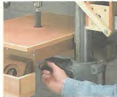
Step 6. Finally, remove the scrap block (see Step 2) and adjust the height of the sanding platform.
