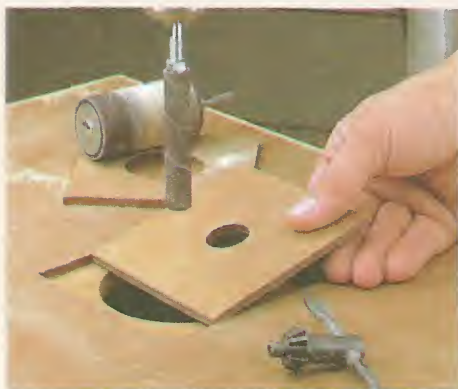
A. Inserts. When you need to change the size of a sanding drum, just slip in an insert with a different size opening.
