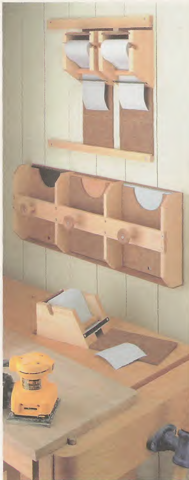
▲ A dispenser for rolls of adhesive-backed sandpaper. And a press for sheets of sandpaper. Build each one as a separate unit or "gang" them together for more storage.
