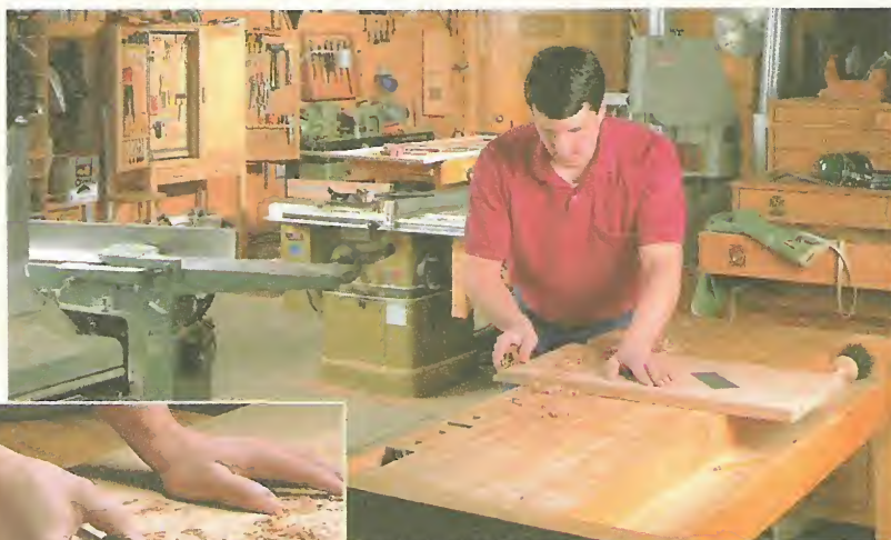
▲ Steve Johnson (our shop craftsman) chamfers the end of a glued-up panel with his Lie-Nielsen low-angle block plane.
