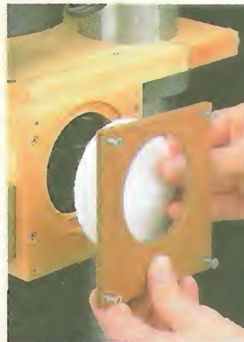
The back of the motor housing encloses an ordinary filter from a dust mask.
