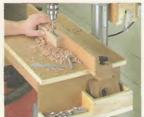
C. Fence. A simple fence with a built-in clamping system also lets you use the sanding platform as a drill press table.
