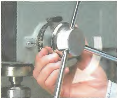
Step 1. Start by setting the depth adjustment for the maximum amount of travel and lock it in place.
