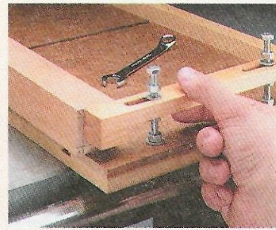
Step 3. Next, align the mark for the taper with the edge of the jig and tighten the adjustment nuts.
