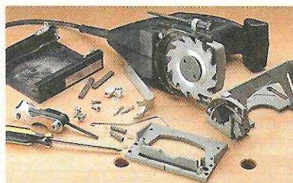
Changing Blades. To provide access to the blade on the Makita, just loosen a knob and flip up the base. But you'll practically have to disassemble the Porter Cable (right) to change blades.
