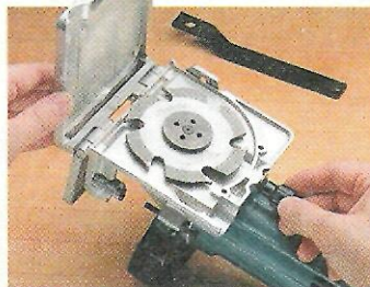
Changing Blades. To provide access to the blade on the Makita, just loosen a knob and flip up the base. But you'll practically have to disassemble the Porter Cable (right) to change blades.
