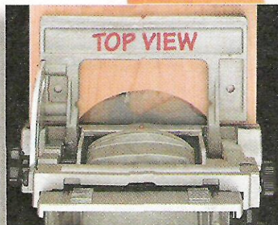
▲ These new plate joiners make it easy to cut the matching curved slots for a biscuit, see photo at left.
