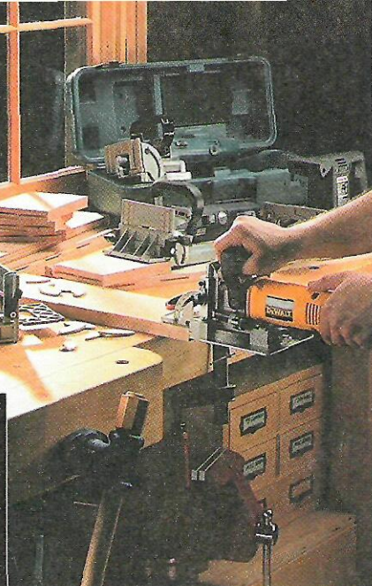
▲ These new plate joiners make it easy to cut the matching curved slots for a biscuit, see photo at left.
