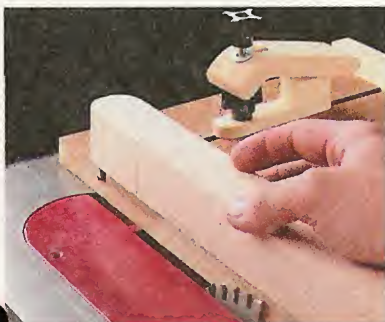
Step 4. Now lay out the starting point of the taper and align the mark with the edge of the jig.
