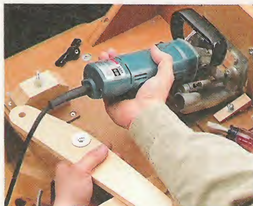
Quick Release. If you want to use the plate joiner in a hand-held position, simply loosen a pair of hold-downs and remove the pivot arm.
