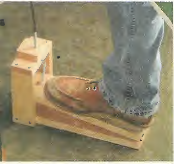
When you "step on the gas" with this foot pedal, it plunges the blade of the plate joiner into the workpiece.
