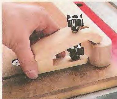
Step 5. Slide the stop against the leg and lock it in place. Then tighten the hold-down on the leg.
