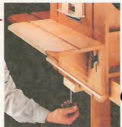
Sliding Table. A built-in height adjustment mechanism raises or lowers a sliding table. This establishes the location of the slot that's cut for the biscuit.
