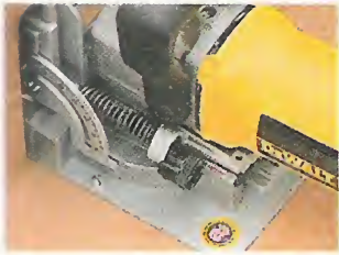
Holes in the base of this DeWalt joiner can be used to screw it directly in place.
